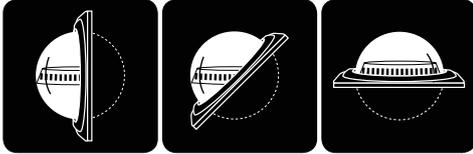
The compass should be positioned where it can be easily read from all angles. Position the compass as far as possible away from iron objects or other disturbing magnetic sources as loud speakers, windscreen wipers, instruments etc.
